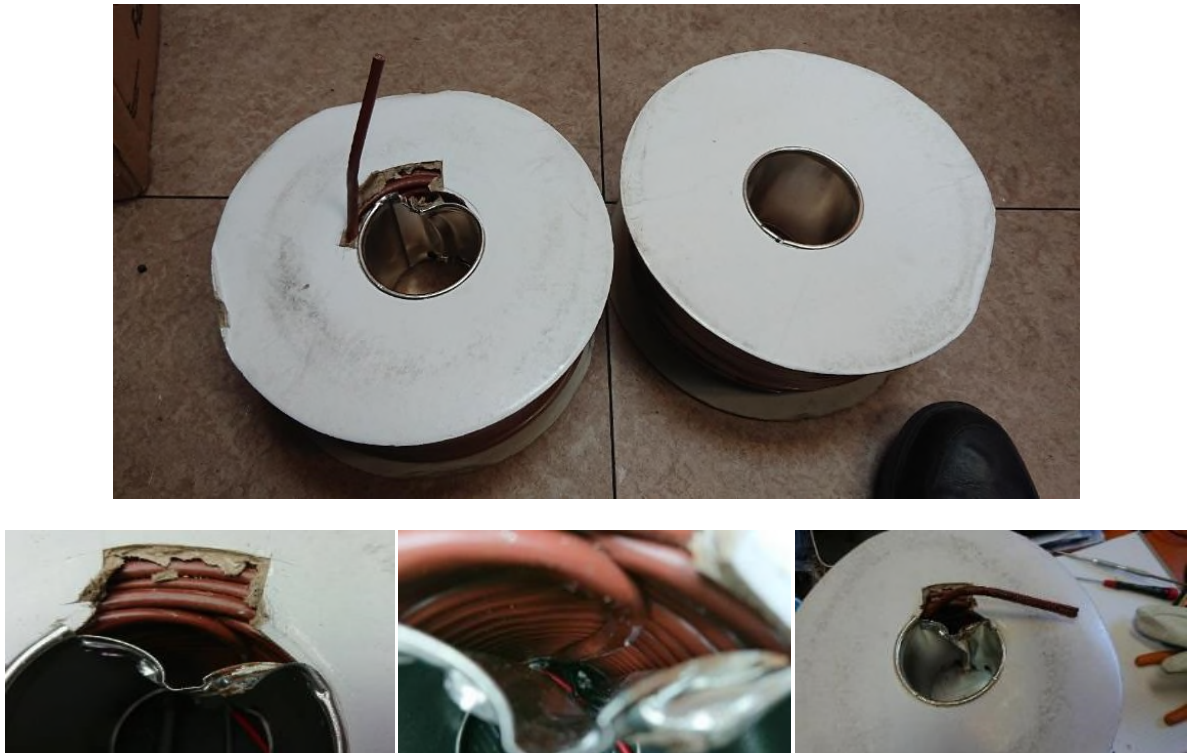
Figure 8 – Extracting Buried End for Splicing Pig-tails
