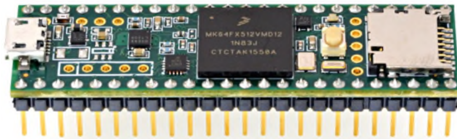
The transceiver is based on the Teensy 3.5 computing module.
