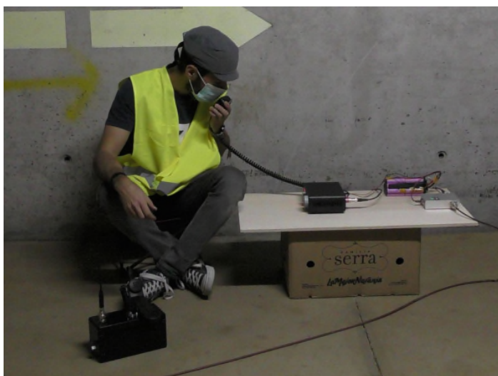
Speech tests in the service galleries at the UC3M campus provided good communication over 800m.
