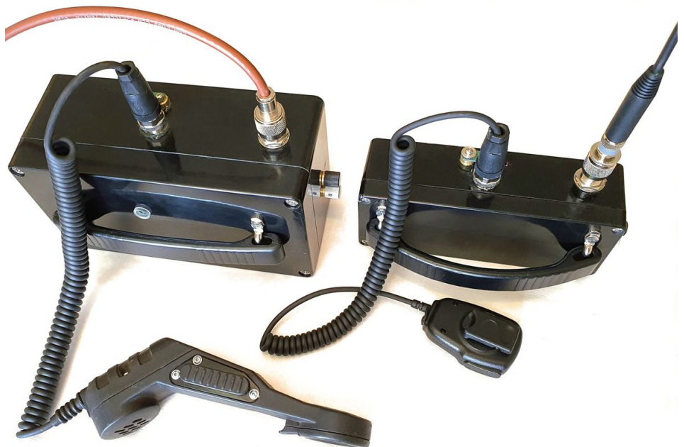
Typical Guidewire Base Station and Handheld Radios These radios were based on off-the-shelf CB radios, re-housed in ATEX enclosures but other options are possible.
