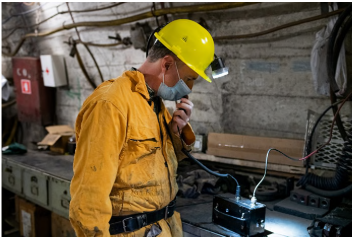
Tests of the guidewire system in the Velenje Coal Mine showed its suitability for rescue communication.
